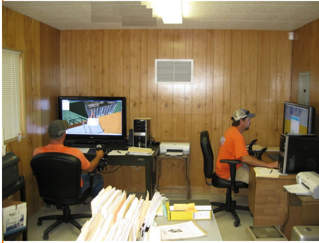
Pictured are 2 of the 5 simulator stations at Local 701's Eugene Training Center where each PC is dedicated to a specific type of equipment, with a combination of OEM, Replica and PC Controls.
