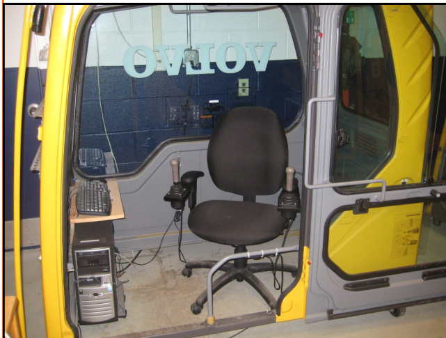
A closer look at the Hydraulic Excavator Personal Simulator with Original Equipment (OEM) joysticks mounted to an office chair inside a real excavator cab.
